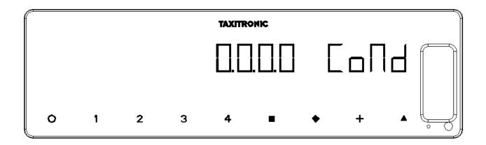
Enter the Driver number changing the numbers using the 1, 2, 3 y 4 keys. Press the key.
