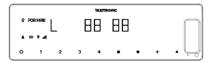
In this case, the bulb lights that are working ok are the 1,2,4 and 5. The bulb light number 3 is not working.
