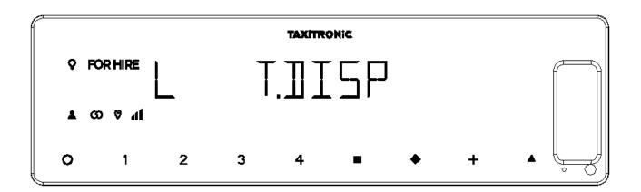
Press key to display the test sequence. (0,1, ...,9).
