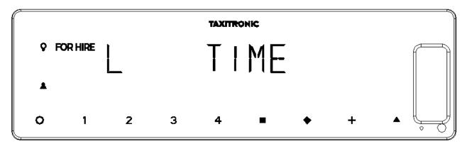
By pressing key if shift control enabled, the remaining time and the available breaks will appear. If the shift control is not enabled, it will directly show the time.
