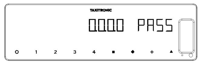
Enter the Password number changing the numbers using the 1, 2, 3 y 4 keys. Press the key.
