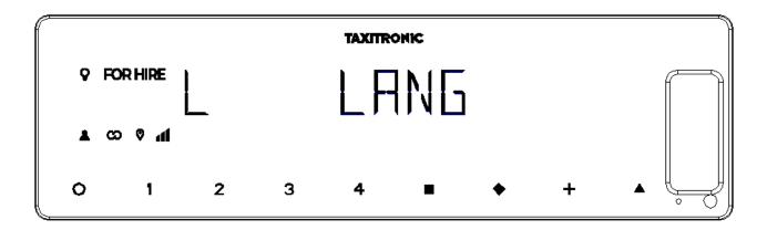
By pressing **O** key or after few seconds it switches to FOR HIRE.
