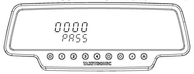
Enter the Password number changing the numbers using the **1**, **2**, **3** y **4** keys. Press the **D** key.
