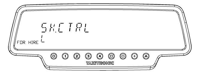
By pressing **O** key or after few seconds it switches to FOR HIRE.
