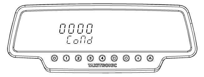
Enter the Driver number changing the numbers using the **1**, **2**, **3** y **4** keys. Press the **D** key.
