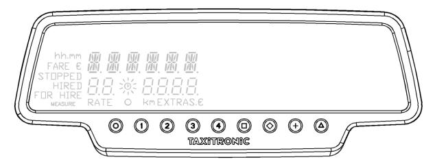
Press the **O** key to turn the Taximeter ON. If a password is required, the second point in the status display will blink, waiting for the introduction of the code.
