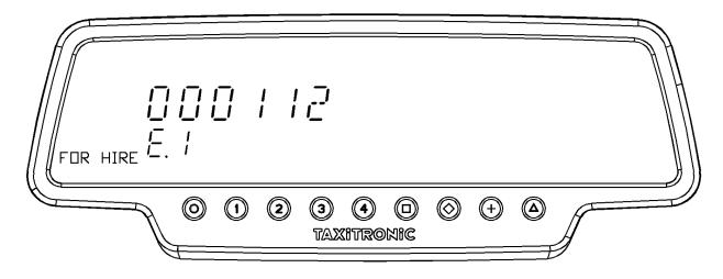
Press **D** key to go to the next visualization, or automatically after few seconds:
