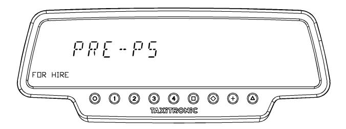
After that time the device enters in the Pause status. The Extras display will show the hours and minutes that the taximeter is in Pause. Pressing the + key the Extras displays shows the total time that the device has been in Pause status. To exit the Pause or Pre-Pause status, the **O** key. It will also exit Pause/Pre-Pause if the car starts moving.
