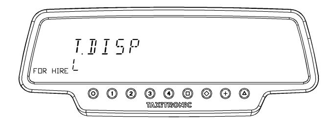
Press key  $\square$  to display the test sequence. (0,1, ...,9).
