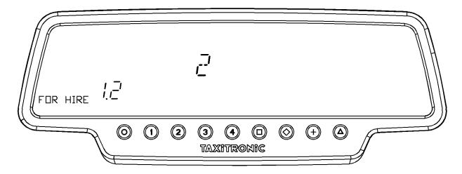
Once the blocks visualization is finished, the taximeter goes to for hire automatically.
