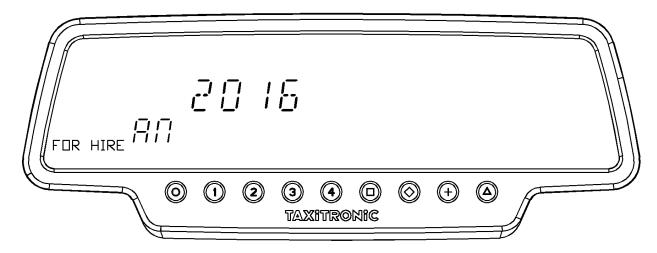
By pressing **O** key or after few seconds it switches to FOR HIRE. **7.4.2.** LIGHT
