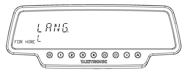
By pressing **O** key or  $\Delta$ , or after few seconds it switches to FOR HIRE.
