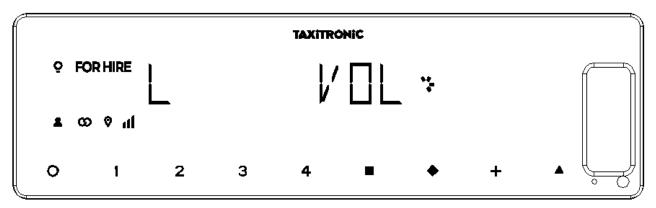
By pressing key to set the volume of the beep. The circular indicator shows the selected intensity.
