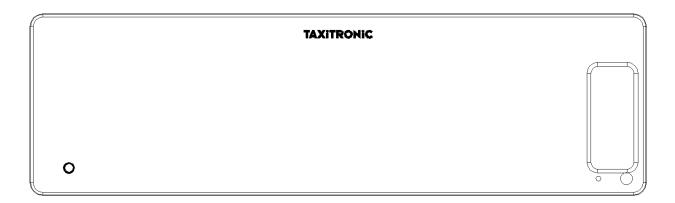
Press the **O** key to turn the Taximeter ON. If a password is required, the second point in the status display will blink, waiting for the introduction of the code.
