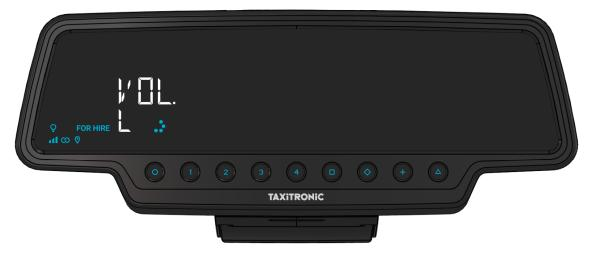
By pressing key to set the volume of the beep. The circular indicator shows the selected intensity.
