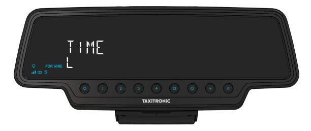
By pressing key if shift control enabled, the remaining time and the available breaks will appear. If the shift control is not enabled, it will directly show the time.
