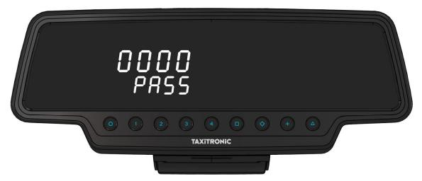
Enter the Password number changing the numbers using the 1, 2, 3 and 4 keys. Press the  $\square$  key.
