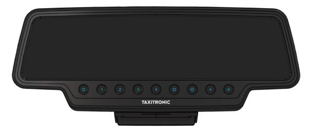
Press the **O** key to turn the Taximeter ON. If a password is required, the second point in the status display will blink, waiting for the introduction of the code.
