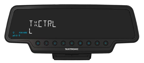
By pressing **0** key or after few seconds it switches to FOR HIRE.
