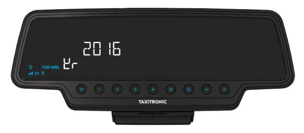
By pressing **0** key or after few seconds it switches to FOR HIRE.
