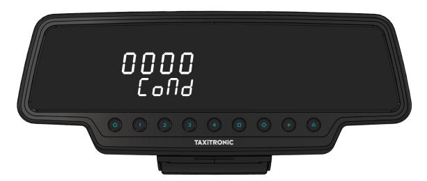
Enter the Driver number changing the numbers using the **1**, **2**, **3** and **4** keys. Press the **\boxed** key.
