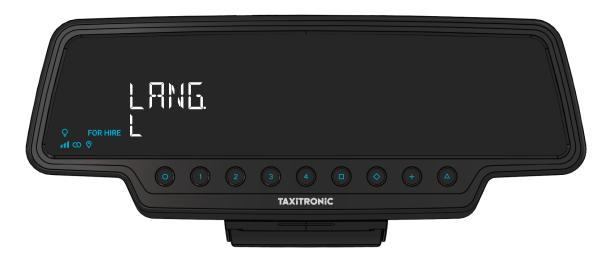
By pressing  ${f 0}$  key or after few seconds it switches to FOR HIRE.
